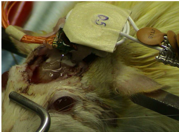
Fig. 6. Wireless in vivo stimulation in the rat motor cortex to wirelessly induce movements in the forelimb.
