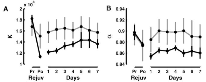
Fig. 3. Voltage biasing caused site-specific, week-long enhancements to electrode conductivity. A representative example from arrays in S1 showed prolonged, reduced levels in both (A) the electrode gain  $K$  and (B) the electrode phase  $\alpha$ . Black traces represent rejuvenated sites in S1 ( $n = 24$ ); gray traces signify nonrejuvenated sites ( $n = 4$ ). Pr: Pre-rejuvenation. Po: Post-rejuvenation. Error bars represent standard errors.
