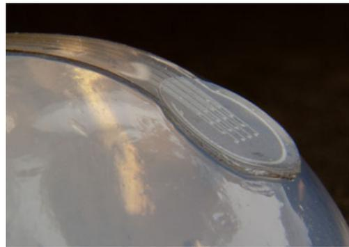
**Fig. 5** An electrode array on a 2 cm-diameter hemisphere of agarose gel (0.5 % w/v) shows that all electrode sites are in contact with the gel surface
