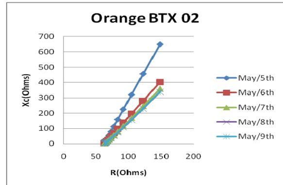
Fig. 6a: Cole-Cole plot comparison of Orange 02 for different days
