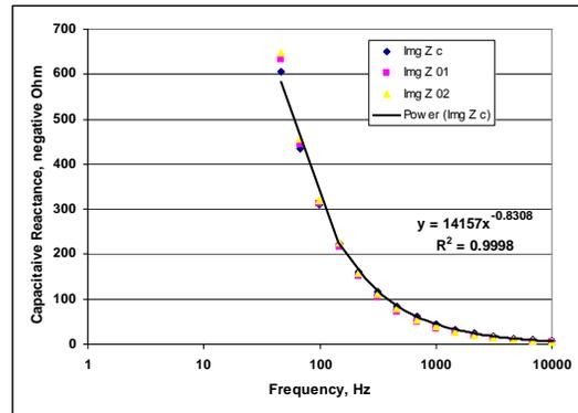
Fig. 4b: Reactance variation with frequency – Fresh orange juice
