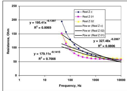
Fig. 4a: Resistance variation with frequency – Fresh orange juice
