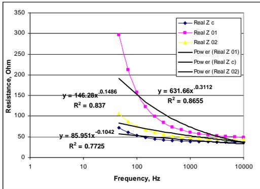
Fig. 3a: Resistance variation with frequency – Fresh Lime juice
