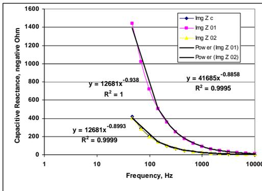
Fig. 3b: Reactance variation with frequency – Fresh Lime juice
