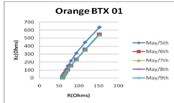
Fig. 6b: Cole-Cole plot comparison of Orange 01 for different days
