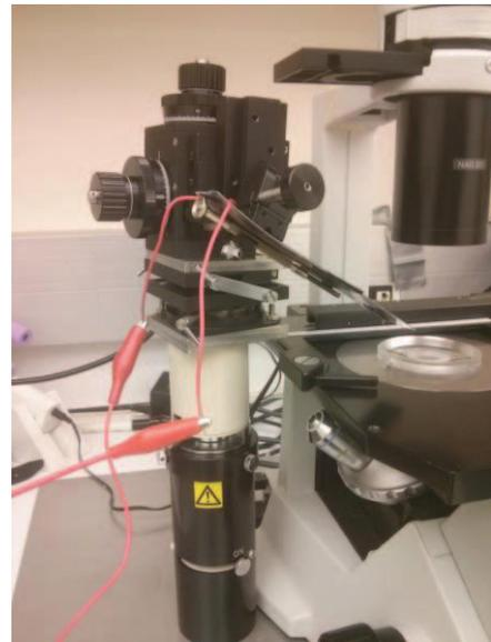
**Figure 3.** A close-up view showing the manipulator system, tungsten electrodes, and a petri dish.
