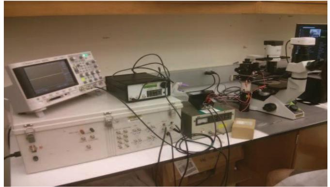
**Figure 2.** Setup showing Oscilloscope, Function Generator, Pulse Generator, HV Power Supply, MicroManipulator and Microscope system
