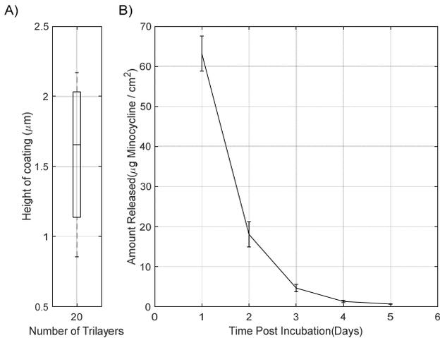
Figure 1. Coating thickness and drug release for verification of coating properties. A) Visualization of the thickness of a 20 LBL coating paradigm on a silicon wafer. B) The drug release from the chips *in vitro* exhibit a similar release profile to that as previously described in literature.
