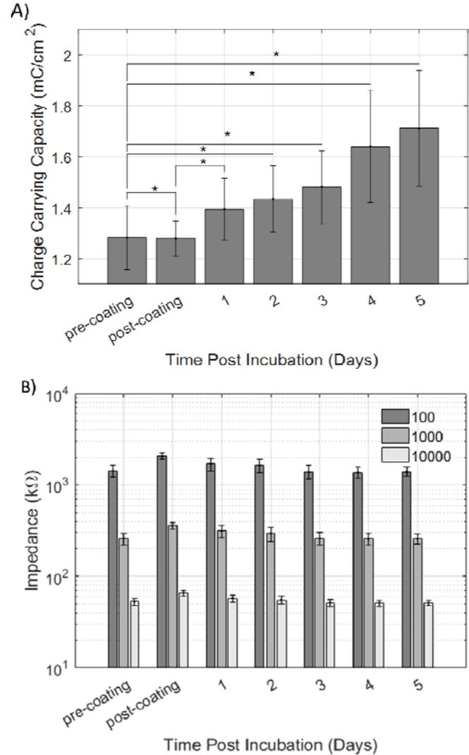
Figure 2. CCC and EIS measurements pre-coating, post-coating, and five days post incubation. A) CCC is initially unchanged after being coated, though increases over the incubation period. B) EIS is initially increased after devices are coated; however, this increase is reduced 1-day post incubation, though significantly higher than pre-coated impedance. Data shown as mean  $\pm$  SEM
